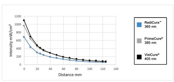
Figure 2. BlueWave® MX-250 Emitter Intensity vs. Distance
