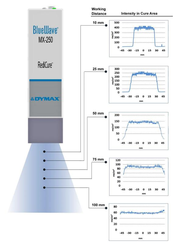
\* Curing area data taken using Fuji UV Light Distribution Mapping System. Output intensity measured using a Dymax ACCU-CAL<sup>™</sup> 50-LED Radiometer in flood-lamp intensity mode.
