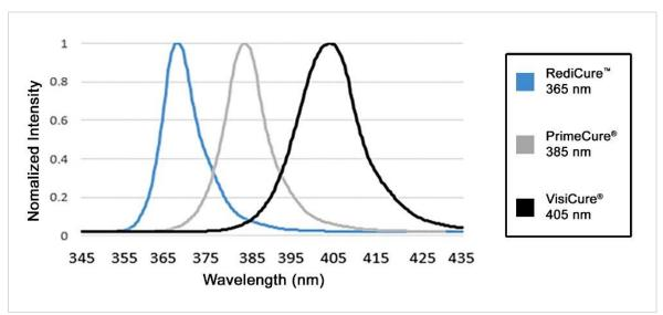
Figure 1. BlueWave® MX-250 Emitter Spectral Output Chart
