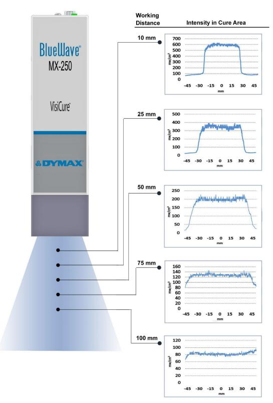
\* Curing area data taken using Fuji UV Light Distribution Mapping System. Output intensity measured using a Dymax ACCU-CAL™ 50-LED Radiometer in flood-lamp intensity mode.
